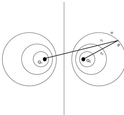
$$(**) \Rightarrow \text{mit Radien} \left\{ \begin{array}{l} r^2 = \frac{k^2}{(k^2 - 1)^2} a^2 \\ r = \frac{k}{|k^2 - 1|} a \end{array} \right.$$
